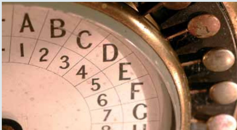
An ABC telegraph of the sort used on overland telegraph systems. Messages were spelled out using the buttons next to the letters.
