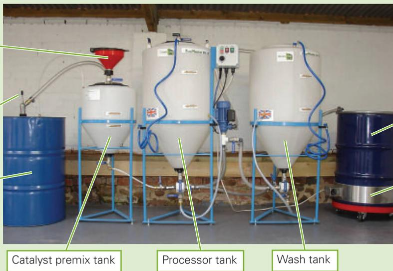
A small-scale biodiesel plant
