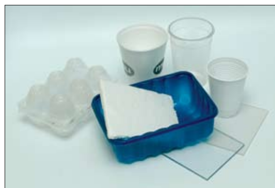
How polymers are processed can make big differences to their properties. All of these items are made from polystyrene.
