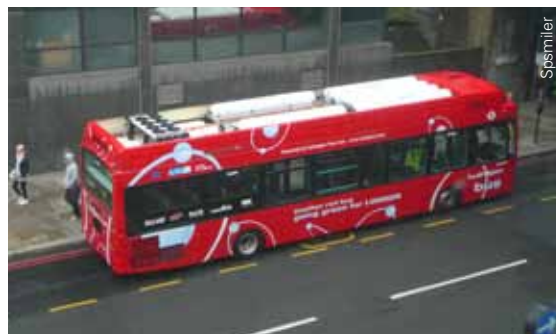
This fuel cell bus travels between some of London's major tourist sites. You can see the six hydrogen fuel tanks on its roof.
