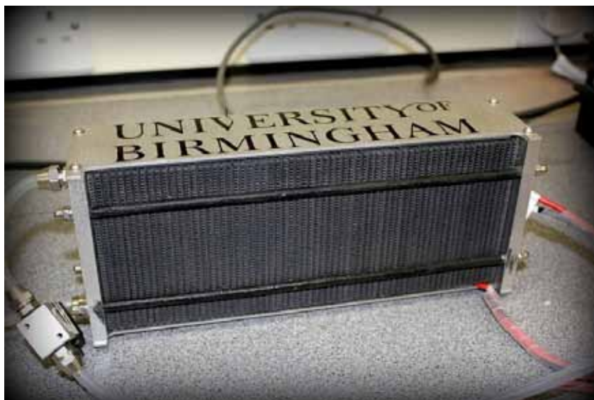
A fuel cell stack, comprised of 64 individual cells. The black tie bars clamp them tightly together to reduce gas leakage from the cells to the environment. Note the gas feed on the left and electrical wires on the right.
