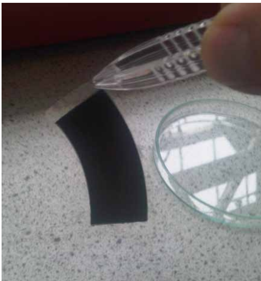
The electrolyte membrane, made of the polymer PTFE. This forms the central part of the fuel cell and allows H + ions to pass through, but not the electrons or gases.
