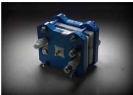
A single-cell fuel cell
