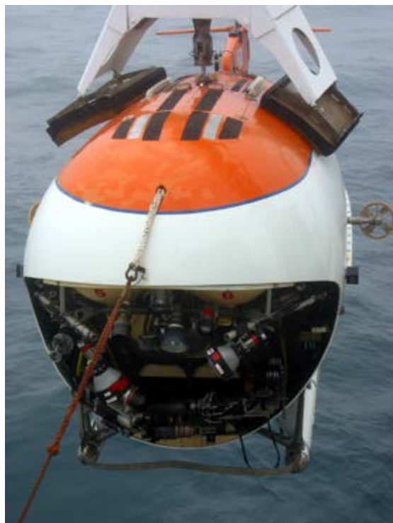
The Mir explorer can reach 6000 m and carry three passengers.
